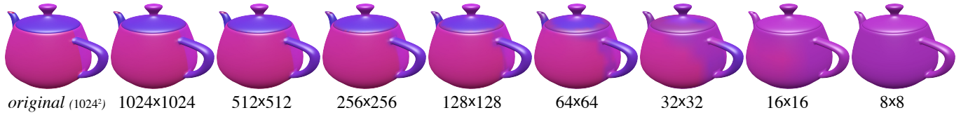
Fig. 6. Decreasing the resolution of a color texture while computing a seam-free texture. The original texture, whose seam runs underneath the handle, is 1024 \times 1024 . This example uses local smoothness parameters (see text for details). As the texture size decreases, the area of influence increases. The change eventually bleeds into the teapot’s lid, a disconnected component. A seam never appears, though at 8 \times 8 resolution, the texture becomes virtually constant.
